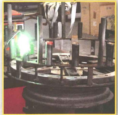
Saldatura gas flux Gas flux welding
